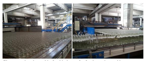
Glass container is used in food industry for food-canning and beverage production. Production capacity of glass jars is 269 mln. pieces at fixed 0.5 l calculation Production capacity of glass bottles is 110 mln pieces at fixed 0.5 l calculation
